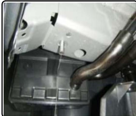
5. Raise the hitch into position. Raise the hitch next to the vehicle tow loop and install the 1/2" carriage bolt through the mounting plate and through the tow loop. Secure the hitch with the 1/2" hex flange nut. Install 7/16" hex flange nuts onto the 7/16" hardware fishwired into position in Step 4.
