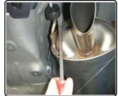
2. Remove the underbody panels from the driver and passenger side rear corners of the vehicle. The panels are held by (3) plastic clips and (2) screws per panels. (1) clip holds the panel to the fascia. The next clip is attached to the frame rail. The last clip is located in the tire well. The first screw is located under the corner of the vehicle. The other screw is on the outside of the tire well. (2) clips will not be reused during the panel reinstallation.
