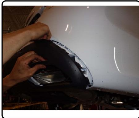
5.) If lowered, raise exhaust and secure back into position.
