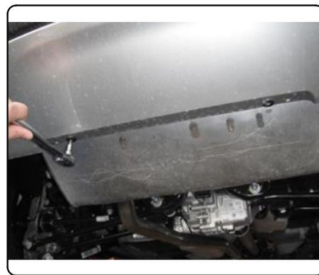
2. Use a 13mm socket to remove the (1) nut on each of the (2) rearward most exhaust hanger brackets. NOTE: Support the exhaust before removing the nuts to prevent damage to the exhaust.
