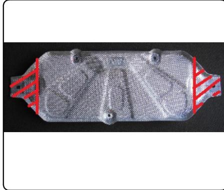
4. Remove the (6) plastic hole covers if present and using a die grinder, enlarge the rearward most holes in the bottom of the frame to allow the supplied carriage bolts and spacers to pass through. Fishwire all (6) 1/2" carriage bolts and CM-SP10 spacers into the mounting positions as shown in the diagram above.
