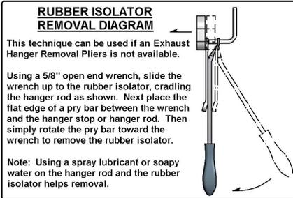
**RUBBER ISOLATOR REMOVAL DIAGRAM**
