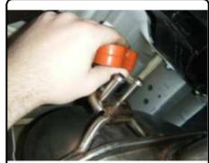
2. Remove heat shield by removing (3) nuts and (1) screw. Trim heat shield to allow hitch side plate to rest against vehicle frame rail. The area trimmed off will remove approximately 8 inches of the heat shield that was along the inside of the frame rail.
