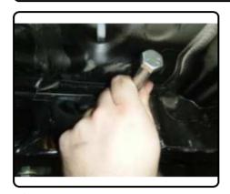
6. Torque 7/16" hardware to 70 lb-ft and M10 hardware to 48 lb-ft. Raise exhaust and spare tire back into position.
