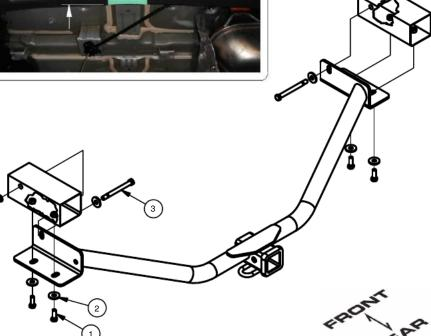
1. Lower exhaust by removing (3) rubber isolators. To ease installation, lower and remove spare tire temporarily.
