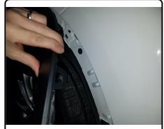
2. Gently unclip (1) reflector on each side of rear fascia to access and remove (1) fastener on each side using 8mm socket.
