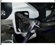
5. Raise hitch into position aligned with vehicle studs and secure using supplied M12 hardware.
