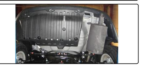
2. Lower exhaust by removing (2) rubber isolators from the hangers attached to the exhaust.
