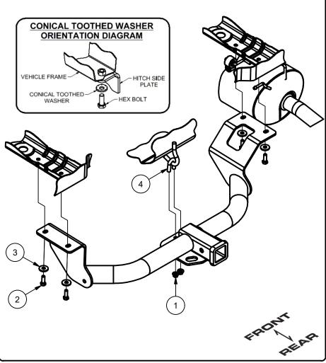
1. Remove (10) fasteners and lower underbody panel.
