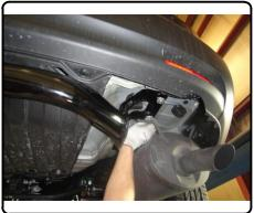
5. Torque all 7/16" hardware to 25 ft-lbs. Torque all 10mm hardware to 48 ft-lbs.
