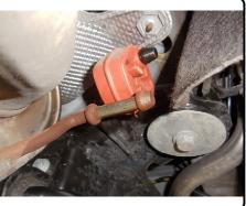
2. Remove rear heat shield at vehicle fascia by removing 4 hex bolts and 8 Torx bolts. Heat shield may either be trimmed and reinstalled or permanently removed.
