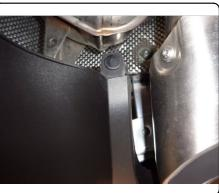
2. Remove lower bumper fascia by lightly pulling along the snap groove, which spans the length of the bumper and disconnect (4) sensor plugs if equipped.Set fascia aside for reassembly.
