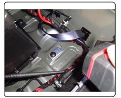
In sequence, torque 1/2" hardware to 110 lb-ft, 8mm bolts to 23 lb-ft, and 3/8" u-bolts to 45 lb-ft. Reinstall lower bumper fascia by following Steps 1-2 in reverse.
