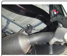
12. Secure hitch and tow loops with supplied 12mm bolts and 1/2" conical toothed washers into weldnuts.
