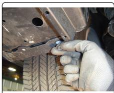
4. Fastener (6) removal. (First photo shows removal technique using flat blade screwdriver.)
