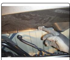
8. Fasteners (12 and 13) removal. Unscrew fasteners, you may need to pull down on plastic to pop fascia free. Remove fascia and place in a safe area. Fascia will be reinstalled in step (17).
