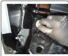
13. Torque all 12mm fasteners to 86 ft-lbs.
