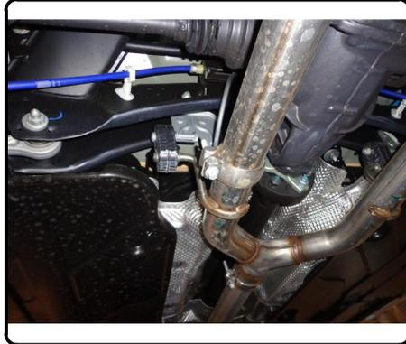
4. Locate plastic fascia support webbing and drill out center inboard section. Enlarge section for 3/4" socket access in order to tighten hitch to nut plates over bumper beam.
