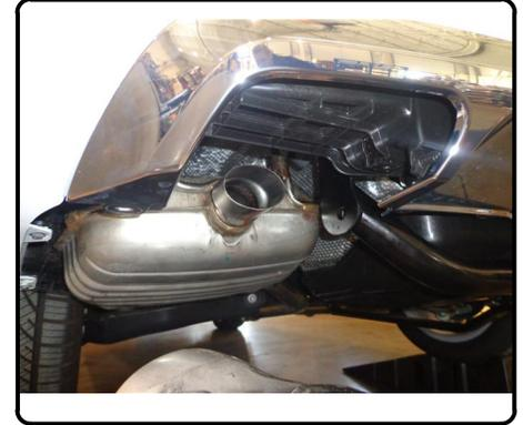
15. Reattach exhaust tip (3 mounting locations each side.)
