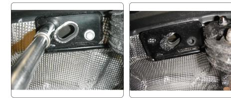
2. Enlarge the access hole to allow 7/16" carriage bolts to pass through on both vehicle frame rails.
