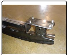
11) Place bumper/hitch on rear of vehicle through original bumper mounting holes. Loosely fasten with the M10 nuts to check fit.
