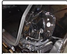
4) Remove (4) M10 bolts for plastic brackets which support the rear fascia, (2) per side. Set aside for reassembly.
