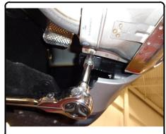
2) Lower exhaust hanger bracket, by removing (2) M10 bolts, (1) per side.
