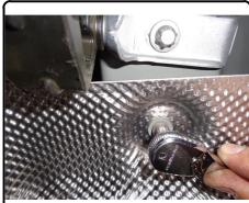
13) Trim heat shield with shears around lower portion of hitch to avoid any contact. Approx. dimensions of cut out should be 1.25" x 4.50".
