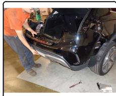
8) Remove (8) M10 nuts on inner panel to remove the bumper, (4) per side. Remove bumper. Set aside bumper and hardware for reassembly.
