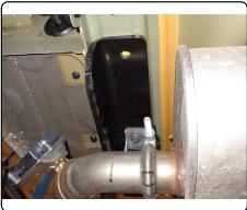
7. Enlarge rearmost hole to approximately 1" on each side of the frame using a die grinder.
