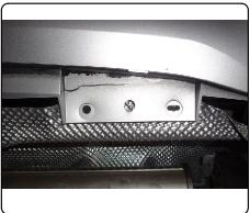
2. Remove (2) M10 bolts for the exhaust brackets. Lower the exhaust.
