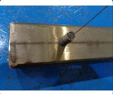
10. Reverse fishwire (1) 1/2" carriage bolt and spacer into the rearmost hole on each frame rail.
