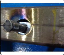
11. Raise hitch into position and pull fishwires so the bolts are in their final position. Remove the fishwires carefully and loosely install the supplied 1/2" hex flange nuts.
