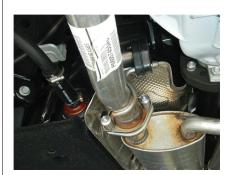
8. Raise exhaust back into position and reattach (2) exhaust isolators. Reinstall (4) exhaust hangers removed in Step 1.
