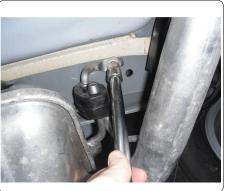
2. Locate and remove (2) rubber isolators from exhaust pipe.
