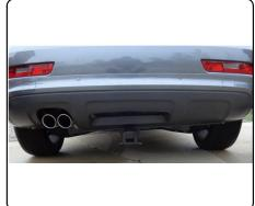
8. Trim a 3-1/2" square section from the center at the bottom of the bumper fascia using aviation shears.
