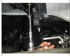
6. Torque all 1/2" fasteners to 110 ft-lbs. Raise exhaust back into position and re-install exhaust hangers.
