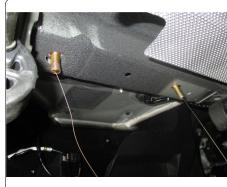
5. Raise hitch into position guiding fishwire ends through attachement holes. Remove fishwires and secure hitch with 1/2" hex flange nuts.
