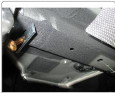
Reverse fishwire one (1) 1/2" carraige bolt and one (1) CM-SP6 through access hole in each frame rail. Leave fishwires attached.
