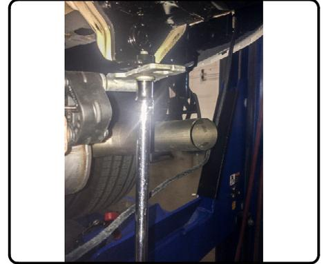
6. Install hitch on rear of vehicle frame using existing studs. Reinstall bumper beam over hitch. Loosely secure M12 hardware.
