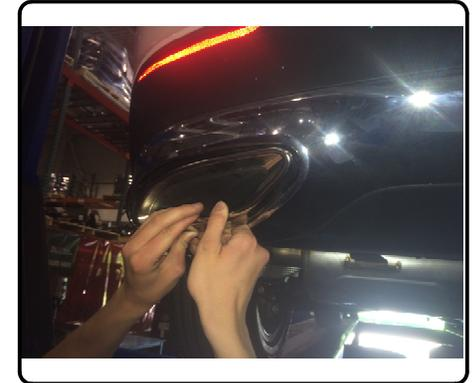
2. Lower exhaust by removing (3) rubber isolators. (As shown in the rubber isolator removal diagram)
