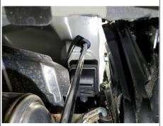
2. On the passenger side, remove (6) M12 bolts using an 18mm socket, to remove tow loop. Return tow loop to vehicle owner. Reinstall emissions canister following step 1 in reverse order.
