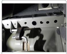
4. Fishwire (2) 1/2" carriage bolts and (2) CM-SP12 spacers through the access hole in the driver side frame rail.
