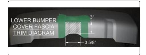
7) Trim the lower bumper cover fascia as shown in the diagram above and reinstall.
