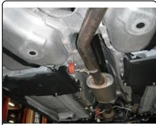
Remove (8) nuts and (10) bolts using a 10mm socket to remove the plastic underbody panel and lower bumper cover fascia.
