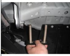
3. Raise hitch into position and slide the bolts through to support it. Loosely install the (4) supplied 1/2" hex flange nuts and the (2) hex bolts and conical washers as shown. Be sure teeth on washers are against the hitch mounting plate.
