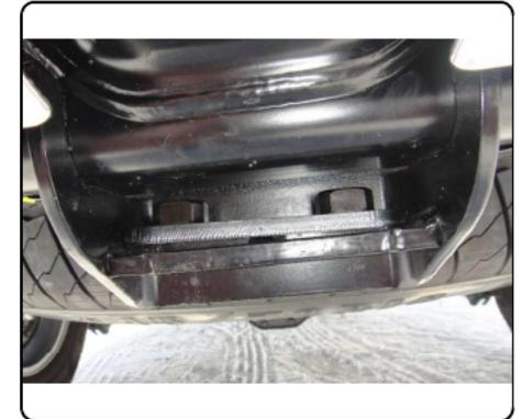
3. Raise hitch into position and loosely secure with 3/4" bolt followed by 1/2" bolt and conical tooth washer.
