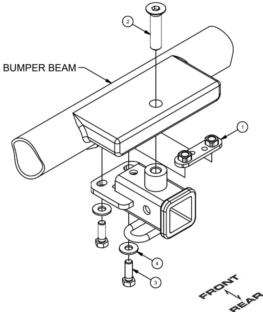
1. Remove plug from center of bumper step and insert 3/4" bolt. Save plug for reinstallation in Step 4.
