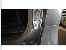
6. Starting from the wheel well and working towards center remove fascia by pulling gently. Be sure to unplug any wires that are attached. Set aside for reinstallation in STEP 11.
