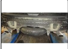
9. Using a hammer, bend bumper mounting flange inward toward the front of the vehicle to allow hitch to mount flush with vehicle.
