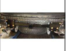
11. Reinstall fascia removed in STEPS 1-6 in reverse order. Be sure to reconnect the plugs that were disconnected during fascia removal process. **Note:** fascia has a removable panel for hitch usage. The panel can then be reinstalled when hitch is not in use.
