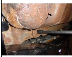
$2. \ \, \text{Move nut plates into location aligned with holes inside frame rail}.$
