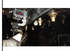
8. Align the driver side bumper bracket with the (2) inside mounting holes on the frame. Secure the bracket to the frame using the long factory M14 bolts removed earlier and (2) M14 hex flange nuts. Repeat on the passenger side.
