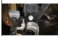
5. Remove (2) factory M6 bolts from the passenger side and (1) M6 bolt on the driver side from the exhaust heat shield. Using a hammer, flatten the heat shield tabs against the frame, heat shield tabs will be pinched between the hitch side plates and the frame.
