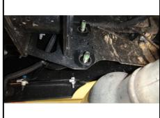
4. Locate and remove the (3) factory M14 bolts on the outside of the driver side frame rail and (1) M14 from the underside of the frame. Repeat on the passenger side frame rail to remove the factory hitch. Save hardware for reinstallation.
