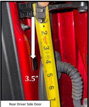
**Step 20:** With the rear driver side sensor attached, you can determine the correct position for the door magnet. peel the backing from the double-sided tape and stick the magnet on the door. Align the bottom of the magnet with the 3.5"
