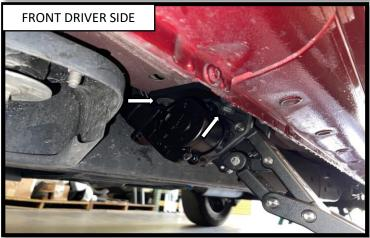
**Step 6**: Install the front driver side motor using ((2) M10x30MM hex bolts M10 Lock Washer, M10 Flat Washer, to fasten the motor to the truck. The hardware should be hand tightened only until snug. This will allow the motor assembly to move and align easier when installing the running board.
