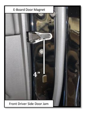
Step 17: FRONT DOOR Apply a vertically oriented strip of masking tape on the front passenger side door using the deepest part of the latch as a reference point. Make a mark 4" below the center line of the latch. Prepare the surface by cleaning with a 50/50 mix of isopropyl alcohol and water or equivalent. Once the surface is completely dry, peel the backing from the double-sided tape and stick the magnet to the door. Align the top of the magnet with the 4" mark as shown.
