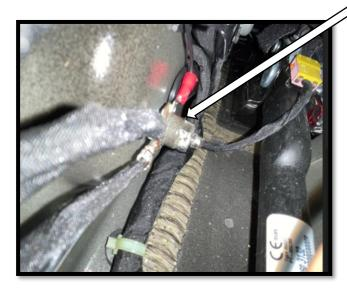
**Step 16:** The door trigger sensor harness will need a ground connection to the vehicle. Locate the seat belt assembly at the passenger side b-pillar and install the ground wire under the top bolt of the seat belt assembly.
