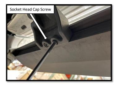
**Step 9**: Determine where you want to position the board and secure the running board to the arms using the (2 per bracket) M6x25 socket head cap screws. Using a torque wrench, tighten to 9 ft-lbs. Step # With the running board is installed, fasten the hardware on the Driver side front and rear motor assemblies. Using a torque wrench, tighten the mounting hardware to 18 ft-lbs.
