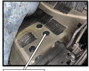
Driver Side Liner, pull back to expose grommet opening
