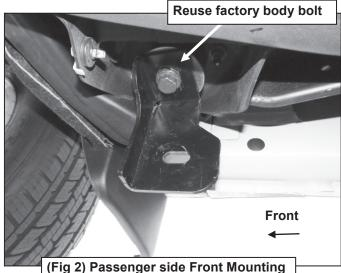
(Fig 2) Passenger side Front Mounting Bracket attached to front body mount
