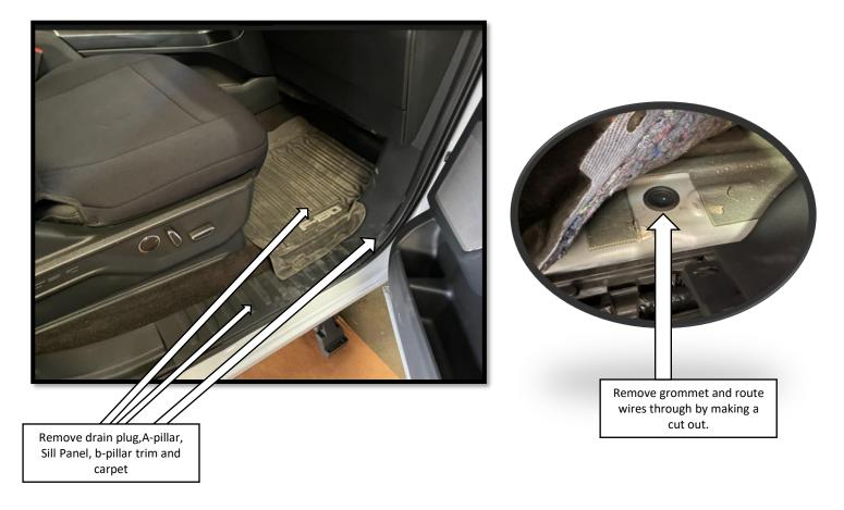
**Step 13:** Go under the vehicle and feed the door trigger signal wires (white and brown) and the disable switch wires (two black wires) into the cab. Feed the wires thru the hole in the rubber drain plug. Pop the grommet back into the slot. Seal around the wires using RTV silicone adhesive to prevent water intrusion.
