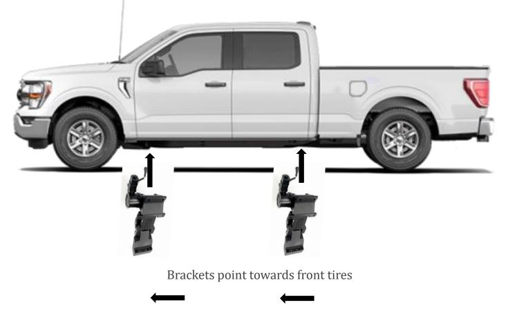
**Step 7**: Repeat Steps 1-6 to install the motor bracket assemblies and running board on the driver side.
