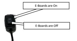
**Step 23:** Open the Driver side door and keep the door open. Flip the disable switch to the Off position. This will signal the running boards to retract to the stowed position and it will disable any further operation until the switch is flipped to the On position.
