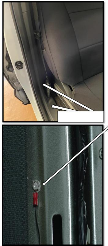
**Step 14:** Route the passenger side door trigger wire (brown) towards the passenger side b-pillar. Route the driver side door trigger wire (white) and the black disable switch wires under the center console to the left side of the vehicle. The white wire needs to go to the driver side b-pillar, the black wires will go to the center console.
