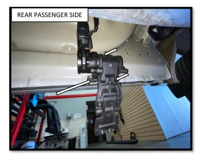
**Step 3**: Install the rear PASSENGER side motor on the 3 threaded studs located on the inside rocker panel towards the rear of cab using (3) M8 Hex Nuts, (3) M8 Flat Washers and (3) M8 Lock Washers. The hardware should be hand tightened only until snug. This will allow the motor assembly to move and align easier when installing the running board.
