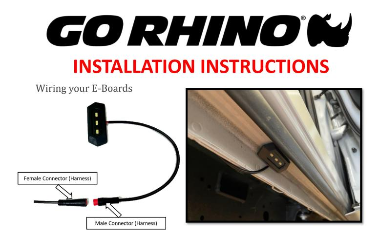
**Step 10**: Align the arrows on the small round connectors and plug the Passenger side front and Passenger side rear LED lights. Prepare the surface by cleaning with a 50/50 mix of isopropyl alcohol and water or equivalent. Once the surface is completely dry, peel the backing from the double-sided tape and stick the LEDs to the bottom side of the rocker panel. Position the LED lights at the center of the front and rear passenger side doors
