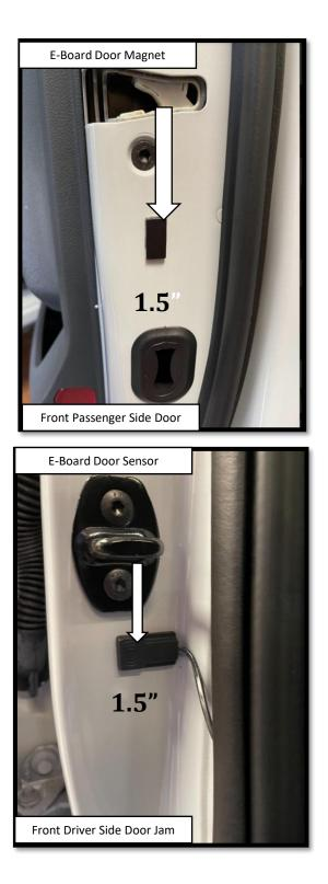
**Step 16: FRONT DOOR** Apply a vertically oriented strip of masking tape on the front Passenger side door using the deepest part of the latch as a reference point. Make a mark 1.5" below the center line of the latch. Prepare the surface by cleaning with a 50/50 mix of isopropyl alcohol and water or equivalent. Once the surface is completely dry, peel the backing from the double-sided tape and stick the magnet to the door. Align the top of the magnet with the 1.5" mark as shown.
