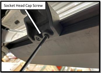
**Step 7**: Determine where you want to position the board and secure the running board to the arms using the (2 per bracket) M6x25 socket head cap screws. Using a torque wrench, tighten to 9 ftlbs. With the running board is installed, fasten the hardware on the Driver side front and rear motor assemblies. Using a torque wrench, tighten the mounting hardware to 18 ft-lbs.
