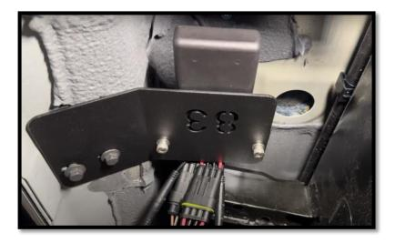
**Step 14:** Go under the vehicle and feed the door trigger signal wires (white and brown) and the disable switch wires (two black wires) and power cables into the cab. Feed the wires thru the hole in the rubber drain plug. Pop the drain plug back into the slot. Seal around the wires using RTV silicone adhesive to prevent water intrusion. These cables will run underneath the driver side seat.
