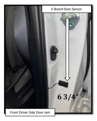
Step 17: FRONT DOOR Apply a vertically oriented strip of masking tape on the front Driver side door using the deepest part of the latch as a reference point. Make a mark 6 3/4" below the center line of the latch. Prepare the surface by cleaning with a 50/50 mix of isopropyl alcohol and water or equivalent. Once the surface is completely dry, peel the backing from the double-sided tape and stick the magnet to the door. Align the top of the magnet with the 6 3/4" mark as shown.
