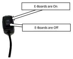
**Step 24:** Open the Driver side door and keep the door open. Flip the disable switch to the Off position. This will signal the running boards to retract to the stowed position and it will disable any further operation until the switch is flipped to the On position.
