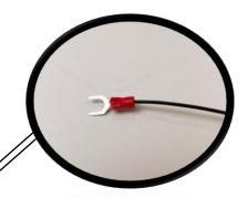
**Step 16:** The door trigger sensor harness will need a ground connection to the vehicle. Locate the seat belt assembly at the driver side b-pillar and install the ground wire under the top bolt of the seat belt assembly.
