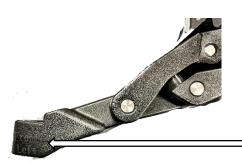
**Note:** Each motor is etched to call out what position it is installed in.
