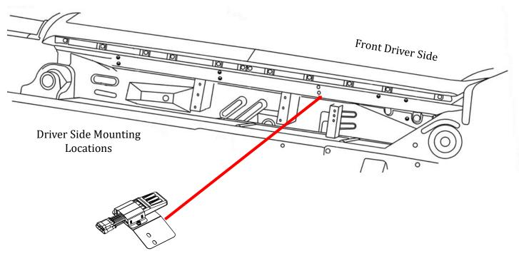
**Step 5**: Install the control module on Driver side using (2) M8X30mm Flange Bolts, to fasten the motor to the vehicle. Use the center rear mounting location. The hardware should be hand tightened only until snug. This will allow the motor assembly to move and align easier when installing the running board.
