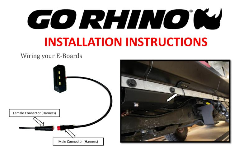
**Step 16**: Align the arrows on the small round connectors and plug the Passenger side front and Passenger side rear LED lights. Prepare the surface by cleaning with a 50/50 mix of isopropyl alcohol and water or equivalent. Once the surface is completely dry, peel the backing from the double-sided tape and stick the LEDs to the bottom side of the rocker panel. Position the LED lights at the center of the front and rear passenger side doors
