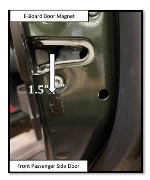
**Step 21: FRONT DOOR** Install front magnet (small) onto the front passenger side door about 1.5" below the center line of the latch. Prepare the surface by cleaning with a 50/50 mix of isopropyl alcohol and water or equivalent. Once the surface is completely dry, peel the backing from the double-sided tape and stick the magnet to the door. Align the top of the magnet with the 1.5" mark as shown. Verify that the magnet should be in line with the door sensor.
