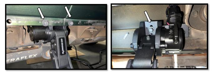
**Step 6**: . Install rear passenger side bracket onto weld seam using (2) M8x20MM Hex Bolts, M8 Lock Washer, M8 Flat Washer. On the underside of the bracket, secure it to the motor to the mounting plate using (1) M8x35MM Hex Bolts, M8 Lock Washer, M8 Flat Washer.
