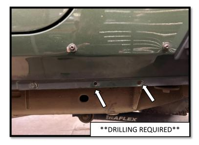
**Step 7**: Using a 21/64" drill bit, chase the two front motor mounting holes on the pinch seam. Use touch up paint to cover up any raw metal on the pinch seam.
