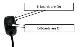
**Step 28:** Open the Driver side door and keep the door open. Flip the disable switch to the Off position. This will signal the running boards to retract to the stowed position and it will disable any further operation until the switch is flipped to the On position.
