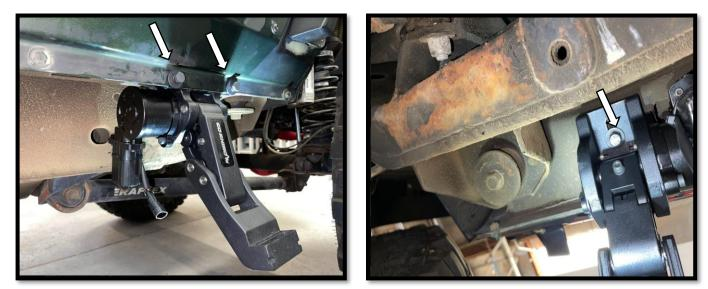
**Step 8**: . Install front passenger side bracket onto weld seam using (2) M8x20MM Hex Bolts, M8 Lock Washer, M8 Flat Washer. On the underside of the bracket, secure it to the motor to the mounting plate using (1) M8x35MM Hex Bolts, M8 Lock Washer, M8 Flat Washer.
