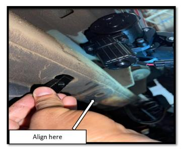
**Step 9**: Locate elongated hole opening on the front of the frame (bottom of the frame) and insert the M12 threaded plate and align thread with hole on the bottom side of the frame.
