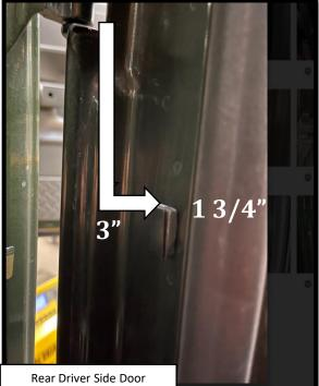
**Step 23: REAR DOOR** Install rear sensor about 1" from the lowest point of the door hinge. Prepare the surface by cleaning with a 50/50 mix of isopropyl alcohol and water or equivalent. Lift the bulb door seal to route the sensor wire underneath it. Once the surface is completely dry, peel the backing from the double-sided tape and stick the rear door sensor to the door jamb as shown.
