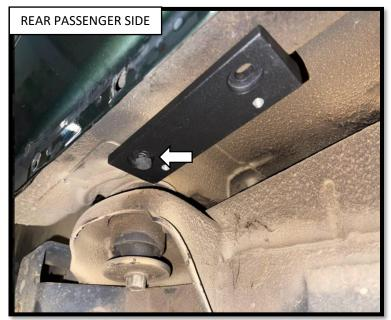
**Step 3**: : Install the rear passenger side motor mounting bracket using an M8 hex head bolt, M8 flat washer and M8 split lock washer. Leave the hardware snug and hand tight.
