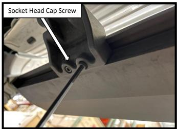
**Step 13**: Determine where you want to position the board and secure the running board to the arms using the (2 per bracket) M6x25 socket head cap screws. Using a torque wrench, tighten to 9 ftlbs. Step # With the running board is installed, fasten the hardware on the Passenger side front and rear motor assemblies. Using a torque wrench, tighten the mounting hardware to 18 ftlbs.
