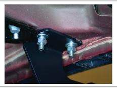
Locate the driver-side middle mounting point. Insert a 60mm T-bolt plate into the opening. Slide a plastic bolt retainer over the thread of the bolt to hold the bolt in place.
