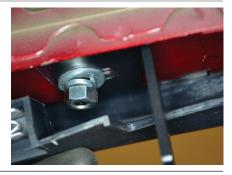
Locate the driver-side rear mounting point. Insert a 60mm T-bolt plate into the opening. Slide a plastic bolt retainer over the thread of the bolt to hold the bolt in place.
