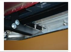
Attach the running board to the brackets using six 8mm bolts, lock washers, flat washers and nuts.
