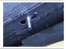
Place an L-shaped hanger bracket onto the vehicle and secure with an 8mm flat washer, 8mm lock washer and 8mm hex nut.
