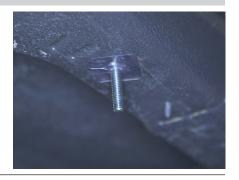
Locate and remove the hole plug in the rocker panel. Insert an 8mm T-bolt plate into the opening. Slide a plastic bolt retainer over the thread of the bolt to hold the bolt in place.
