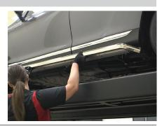
Attach the running board to the brackets using six 8mm bolts, six 8mm nuts, six 8mm lock washers and six 8mm flat washers.
