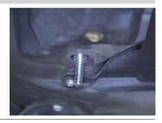
Place the front driver side bracket onto the vehicle and secure with two 10mm hex nuts, two 10 mm lock washers and two 10mm flat washers.
