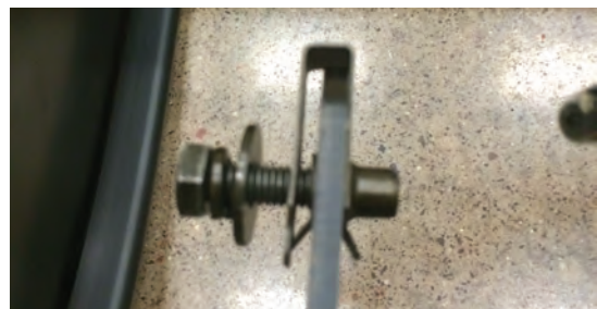
(Fig 12) Insert an 8mm clip nut over the end of the support flange and insert an 8mm hex bolt
