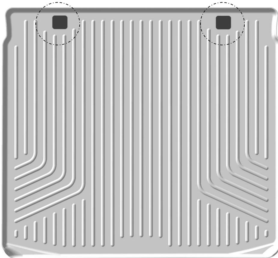
TO ACCESS THE CARGO TIE-DOWN HOOKS WITH YOUR LINER IN PLACE, SIMPLY TRIM THE MATERIAL FROM THE TWO LOWERED AREAS (SHOWN ABOVE CIRCLED/DARKENED). THE LOWERED EDGE IS THE TRIMMING GUIDE. A UTILITY KNIFE OR SIMILAR WORKS WELL FOR TRIMMING.
