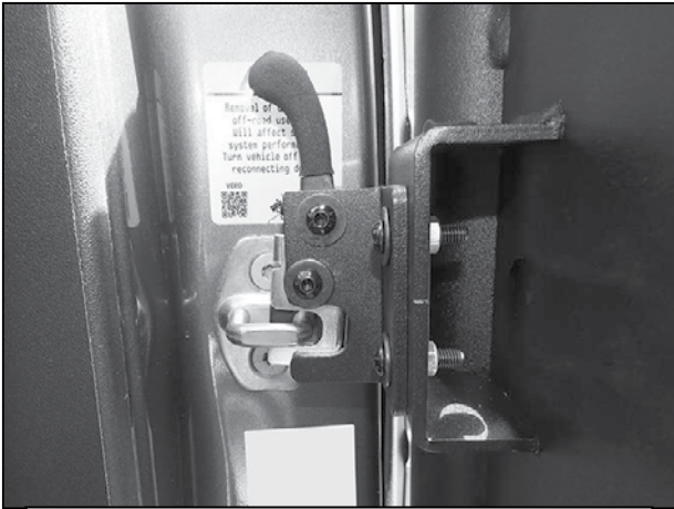
(Fig 14) Make sure door latch fully closes against striker before tightening hardware
