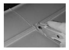
3. Where applicable, feed the strap through the liner that used to lower your third row seats. Vehicles with power folding rear seats will not have the straps.
