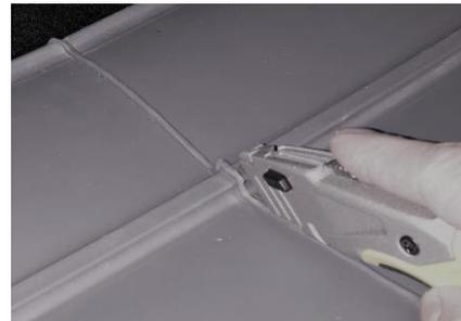
3. To access the LATCH attachment points on the back of the larger 3<sup>rd</sup> row seat back, you will need to trim your liner. Use the recessed trough around the inside bottom of the opening. A utility knife works well for trimming.
