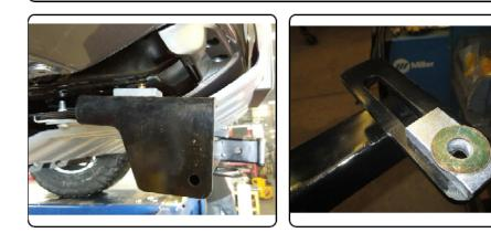
4. Insert one (1) M12 hex bolt with one (1) 1/2" conical toothed washer through side plate, CM-SP52 spacer and 1/2" flat washer into each rear most weldnut.
