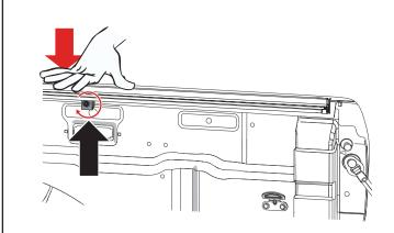
FOR TRUCKS WITH CARGO RAILS: Insert the second clamp (D) above the cargo rail near the tailgate. Slide the second clamp to approximately the center of the rail. Hand tighten the bolt enough to hold the clamp in place.
