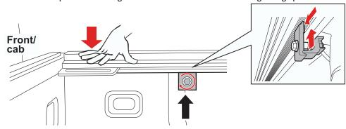
Place the second clamp (D) near the center of the rail.
