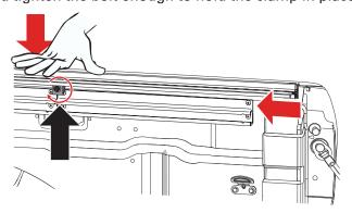
Place the third clamp (E) near the rear of the rail, approximately 12" from the tailgate. Hand tighten the bolt enough to hold the clamp in place. FOR TRUCKS WITH CARGO RAILS: The rear clamp should be positioned as shown here, at the end of the cargo rail on the tailgate side.
