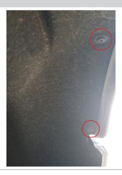
Pry off fenders to access the filler panel clips removing any necessary bolts.
