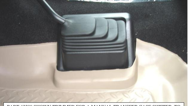
PART #3389 SHOWN TRIMMED FOR A MANUAL TRANSFER CASE SHIFTER. TO TRIM, SIMPLY REMOVE THE LOWERED SECTION ON THE LINER.
