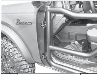
(Fig 9) Adjust fit of Cover and fully tighten all hardware
