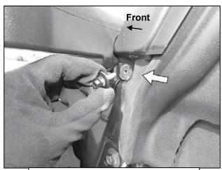
(Fig 2) Remove top fender bolt below/behind outside mirror (arrow)
