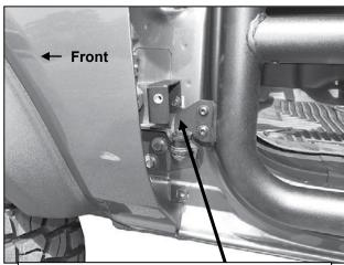
(Fig 4) Reuse the factory hex bolt to attach the driver/left Front Mounting Bracket
