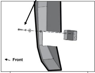
(Fig 8) Attach bottom of driver/left Front Cover to Front Mounting Bracket
