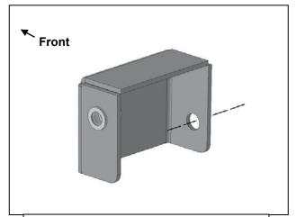
(Fig 3) Driver/left Front Mounting Bracket
