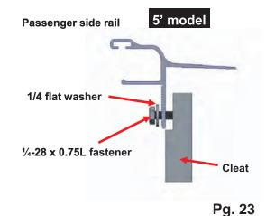
Continue with standard instructions through step 6 (pg. 5) DISREGARD STEP 5, then refer back to this guide on how to install and adjust the mounting hardware.
