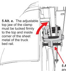
5 Atl. f. If the jaw does not contact firmly into the corner of the bed flange, remove the clamp and loosen the screws to adjust the jaw.
