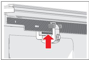
Position the clamps between the adjustment screws. Using a 9/16" wrench, tighten the clamps. It is important to push down on the rail while tightening, AND to tilt the rail up approximately 2 degrees simultaneously. Both the pushing down and tilting of the rail will position the rail best to minimize water intrusion.
