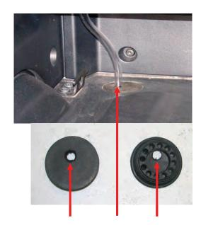
You can pass the tubes through the 2 factory plastic bed bolt covers. Remove the covers and drill a loose ½" hole or a 9/16' hole for the tubes. Offset the holes as shown.
