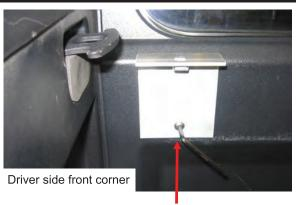
Install front mount brackets as shown. Slide lock washer onto M6 x 40mm bolt, push bolt through hole in mount bracket and start threading into front holes in the bed. **Hold mount bracket level** and tighten using the 4 mm Allen wrench (included). Repeat on passenger side.
