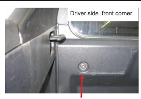
Remove the factory bolts from both corners of the front wall of the bed. Use #40 Torx bit. (included)
