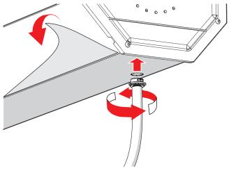
**9c.** Generally the drain tubes will be routed out through a hole drilled in the factory bed plug. Otherwise a suitable existing hole must be utilized. Or a new hole can be drilled, taking great caution to be aware of lines and anything behind where the hole is drilled.
