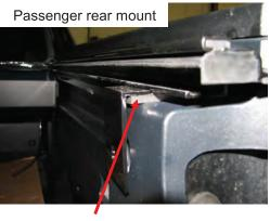
The rubber spacer provided can be added under the passenger rear mount bracket for proper clearance over factory tailgate protector.
