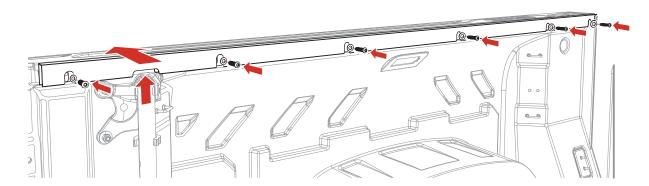
Before tightening the hardware, make sure the top of the CarbonPro rail is level with the top of the plastic bed rail cap.
