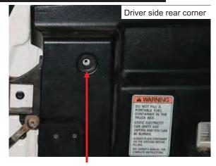
Remove factory screws and spacers from both rear posts using #40 Torx bot. Driver's rear corner is shown.
