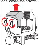
Re-tighten screws and fully engage the lock washers.
