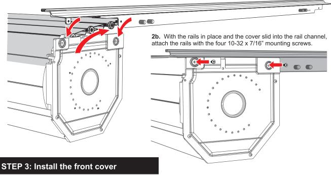
Slide the front cover under the rails, attaching it with the two 10-24 x 3/4" screws and the Allen wrench.
