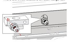
Before tightening the hardware, make sure the top of the Ram Box rail is level with the top of the plastic bed rail cap. Do this on the driver and passenger side.
