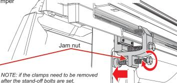
after the stand-off bolts are set, the jam nut and bolt will have to be loosened.
