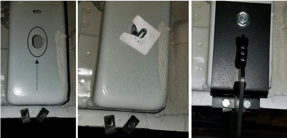
Continue along the side of the vehicle to the 5th mounting bracket repeat steps 3, 4 for the lower mounting holes.
