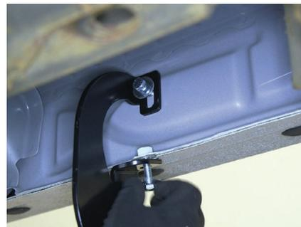
**2B** - Some models will require the use of an 8mm clip nut for the bottom mount location if the vehicle is not supplied with the threaded mount.
