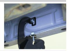
**2B** - Some models will require the use of an 8mm clip nut for the top and bottom mount location if the vehicle is not supplied with the threaded mount.
