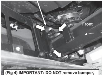
(Fig 4) IMPORTANT: DO NOT remove bumper, ONLY slightly loosen bumper to install Support Brackets. (Passenger/right side frame pictured)
