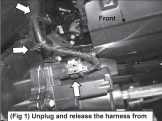
the plastic clips to remove active air dam
