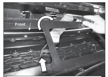
(Fig 9) Pull the Bracket towards the rear of the vehicle and push the front of the Bracket up towards the plastic trim on the bumper
