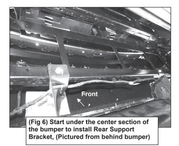
IMPORTANT: Installing the Rear Support Brackets will require multiple movements of the Bracket to get to the mounting location.
