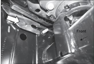
(Fig 12) Place (1) 12mm x 29mm Spacer Washer over the stud in the frame. Slide the Bracket over Washer
