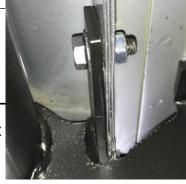
**Step 10.** Next, tighten the remaining hardware that attaches the bracket to the upper body mount.
