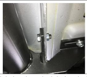
**Step 9.** First, tighten all the hardware that attaches the bracket to the pinch weld of the vehicle.
