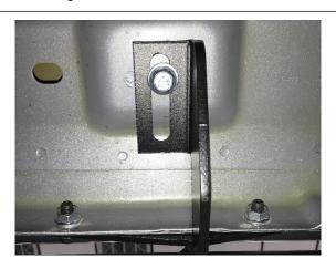
**Step 11.** After finial adjustment, tighten brackets at the main tube.
