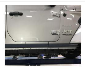
**Step 4.** Carefully raise step up into position and align the brackets with the factory mounting points with the horizontal part of the bracket on the outside of the pinch weld.
